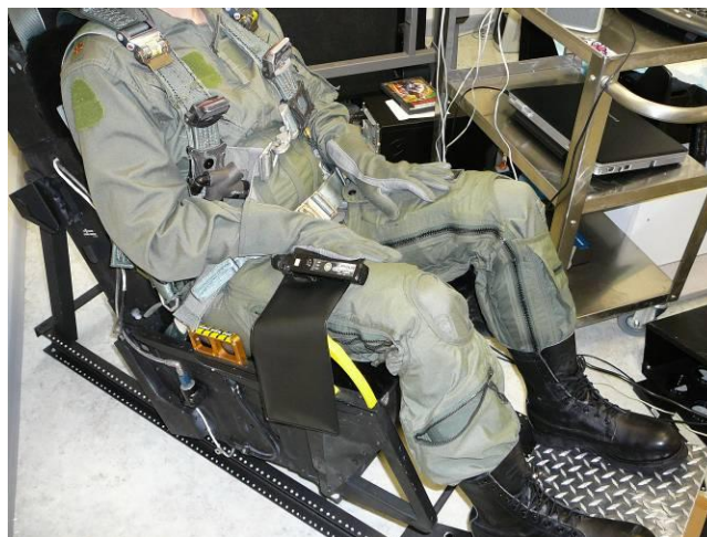
Case study subject testing the AMXDmax System in environmental chamber temp -10C to 55C
